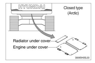
For prevention of overheating in the case of hot ambient air conditions, it is recommended to change covers those have sufficient ventilation area.
